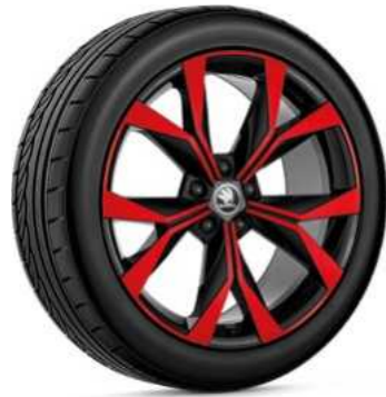
Cetus light-alloy wheel black metallic, red 8.0J × 19" ET45 for 225/40 R19 (4×2), 225/45 R19 (4×4) 57A 071 499E QXJ 57A 071 499AB QXJ*
