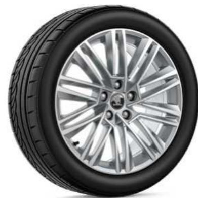
Luxon light-alloy wheel silver metallic brushed 7.5J × 18" ET48 for 225/45 R18 5E3 071 498B 8Z8 5E3 071 498AF 8Z8*
